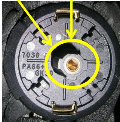
9. Put the actuator back on the 3-way valve and tighten the screw
