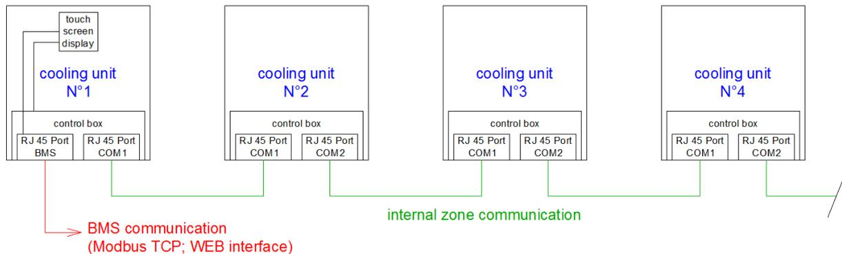
Each controller includes RS485 connector for easy BMS communication via ModBus RTU (a protocol allowing both continuously reliable and accurate remote control of the air-conditioning units) and a port for SNMP card (pCO Web).
