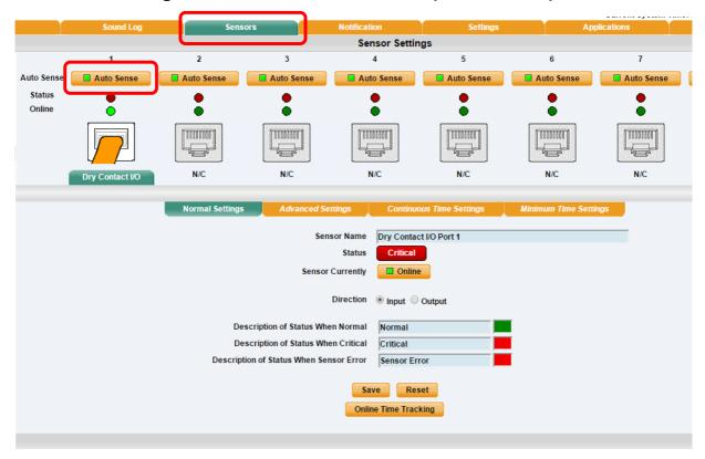
When you first connect the Smoke Detector to the RJ45 port is will be auto sensed online as a Dry contact I/O type sensor. Click the Auto Sense button as shown in the screen shot above.
