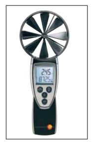
Propeller-type flow meter, diameter 100mm
